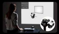
**Projector Profiling** – rotate the ambient diffuser arm to use as a tabletop stand for device positioning, or use the built-in threaded tripod mount for larger venues.
